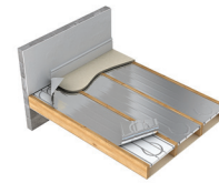
THE BETWEEN-JOIST SYSTEM
