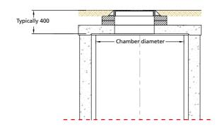
Typically, a standard cover and frame build-up is 400mm with a concrete cover slab, two courses of brickwork and a cover and frame.
