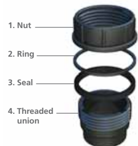
Screw-threaded joint.
